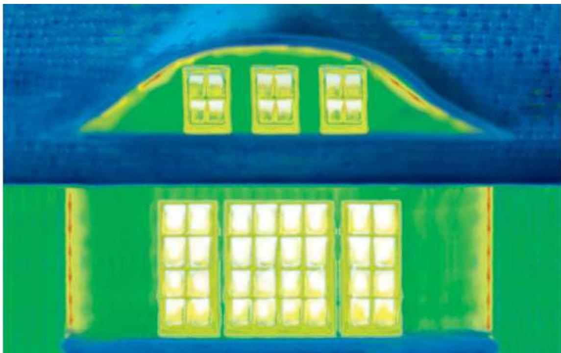
After the renovation: NORDIC DESIGN PLUS windows minimize heat energy losses.
